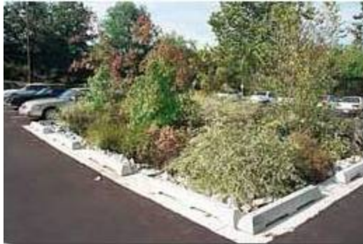
Figure PTP-10- 4 Bioretention System
